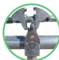
Locking Yoke / Feeding Panel Control Mechanism
